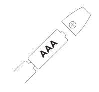
Open the tail cap twisting counter-clockwise, insert a quality AAA battery
